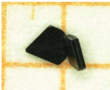
Figure 1. Crystals of \kappa -[(BEDT-TTF) 2 ][Cu(N(CN) 2 )Br] ( 1 ) obtained by the electro-oxidation of BEDT-TTF with the molar electrolyte ratio [Ph 4 P][N(CN) 2 ]:CuBr of 1:1.
